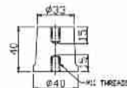
DETAILS OF SUPPORT INSULATOR FOR NEUTRAL BUS BAR (2 Nos.)
