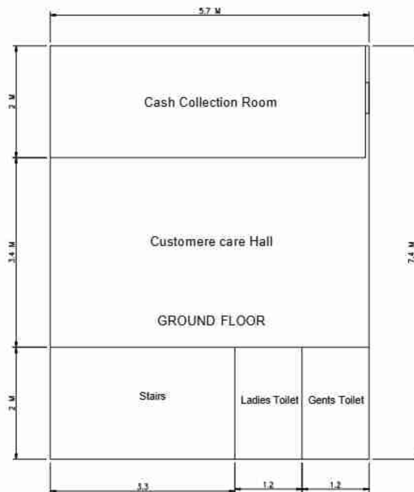
Proposed Double story Control Room Layout plan of 33 /11 KV substation in CITY/TOWN ZONE
