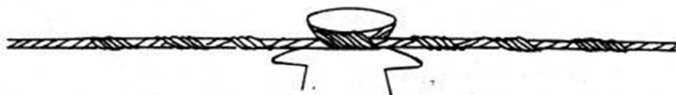
SIDE TIE IN POSITION ON 11KV. PIN INSULATOR
